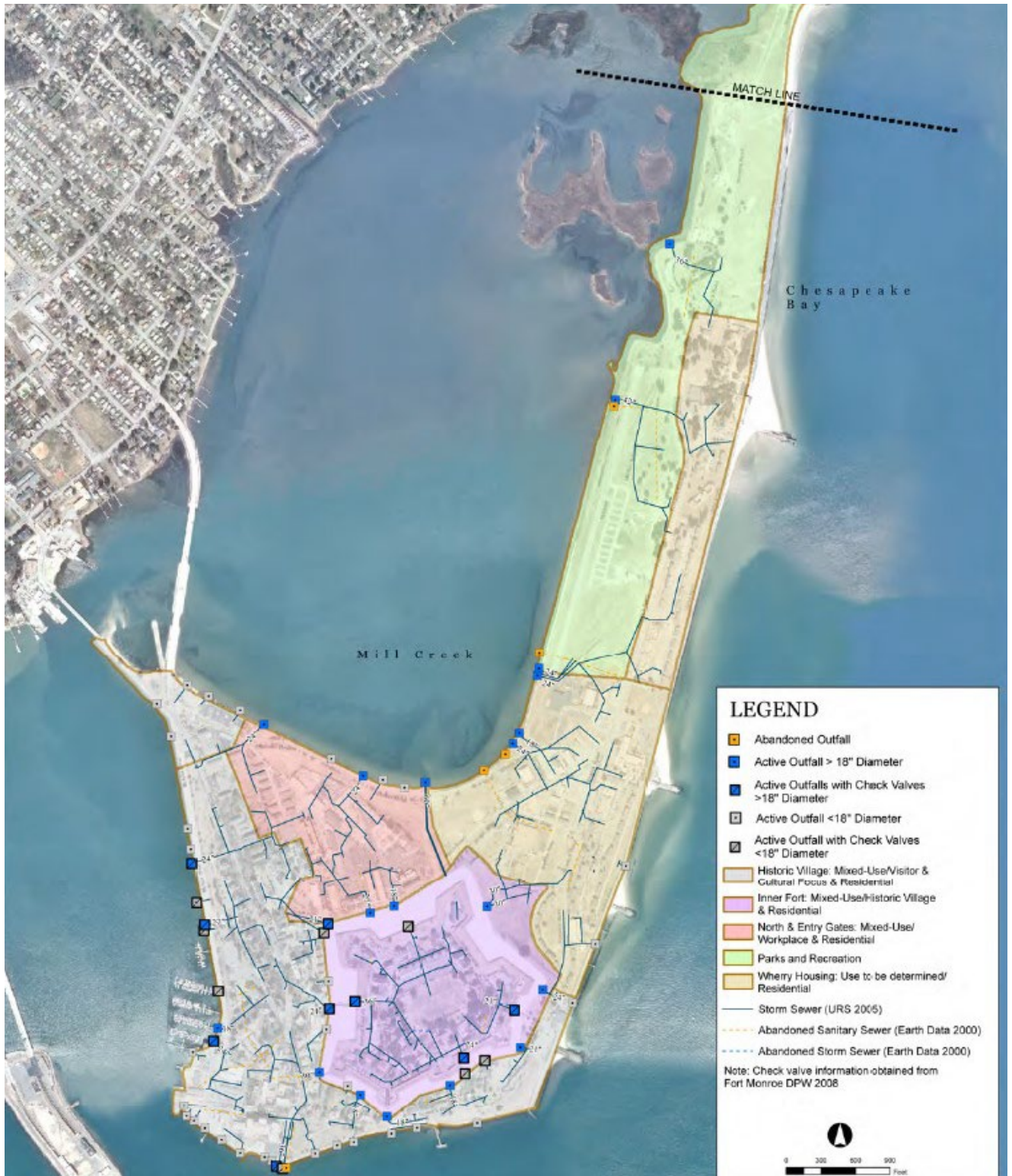
Figure 11: Storm Sewer Lines and Outfalls
